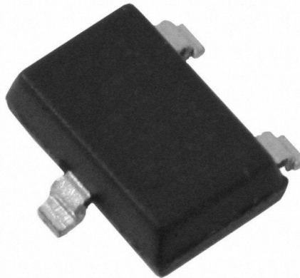
Figura 116 Chips del sensor Hall A3212ELHLT-T (32)
