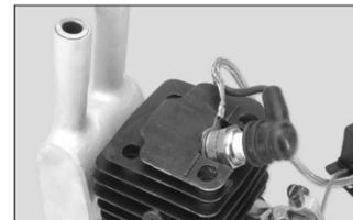
Next, plug the ignition wire from the engine into the matching ignition wire from the ignition module.
