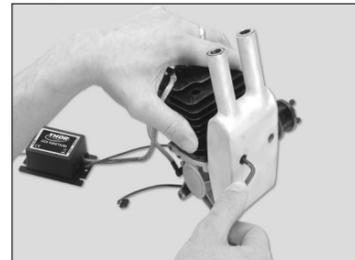
The silencer is mounted to the engine using the two steel socket-cap screws, two spring washers, two square retaining nuts and the gasket provided. Also make sure to tighten the screws firmly. Notice that the nuts slide behind the muffler mounting flange on the engine.
