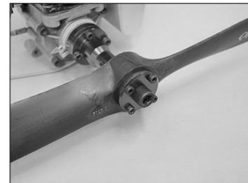
Remove the retaining nut and propeller washer, then drill four 4mm (5/32") diameter holes through the propeller. If you have one, we suggest using a drill press to drill these holes.
