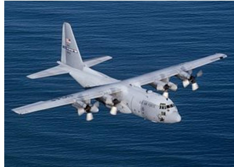
$$\begin{aligned}W_e &= 34400 \text{ kg} \\MTOW &= 70300 \text{ kg} \\S &= 162,1 \text{ m}^2\end{aligned}$$
