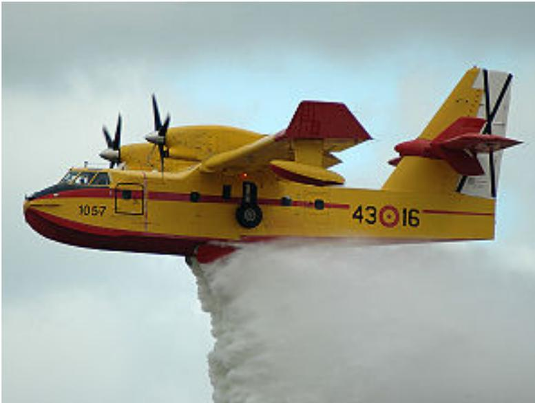
$$\begin{aligned}W_e &= 12065 \text{ kg} \\MTOW &= 19730 \text{ kg} \\S &= 100,3 \text{ m}^2\end{aligned}$$
