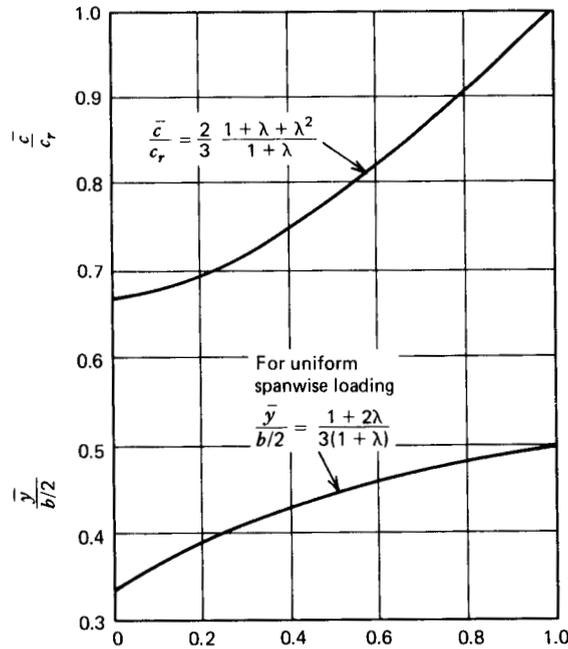
Figure C.2 Mean aerodynamic chord for straight tapered wings; and spanwise position of mean aerodynamic center for uniform spanwise loading (i.e., constant  $C_{L\alpha}$ ). (From "Notes on the Mean Aerodynamic Chord and the Mean Aerodynamic Center of a Wing" by A. H. Yates, *J. Roy. Aero. Soc.*, June 1952.)
