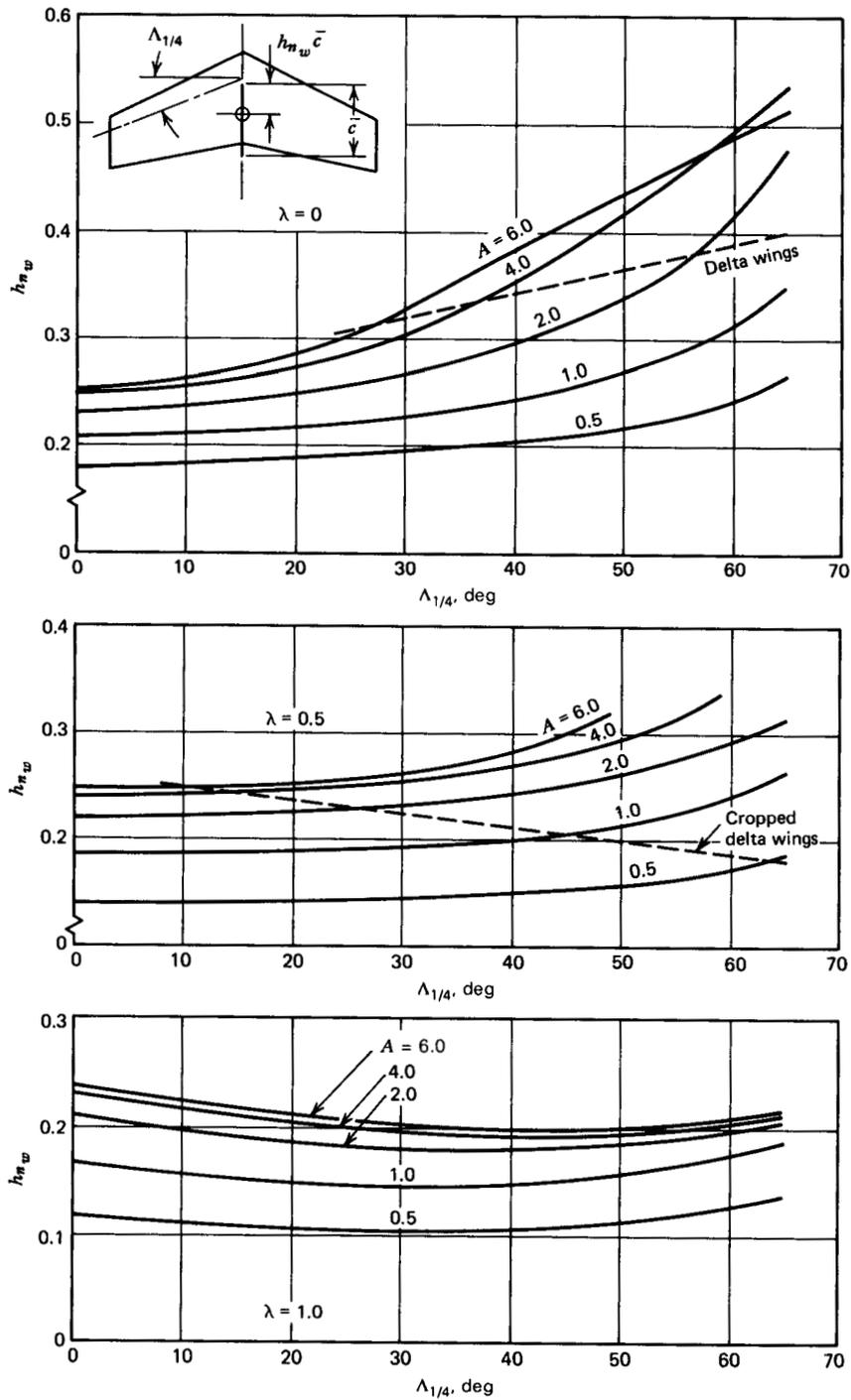
**Figure C.3** Chordwise position of the mean aerodynamic center of swept and tapered wings at low speeds expressed as a fraction of the mean aerodynamic chord. (From Royal Aeronautical Data Sheet Wings 08.01.01.)
