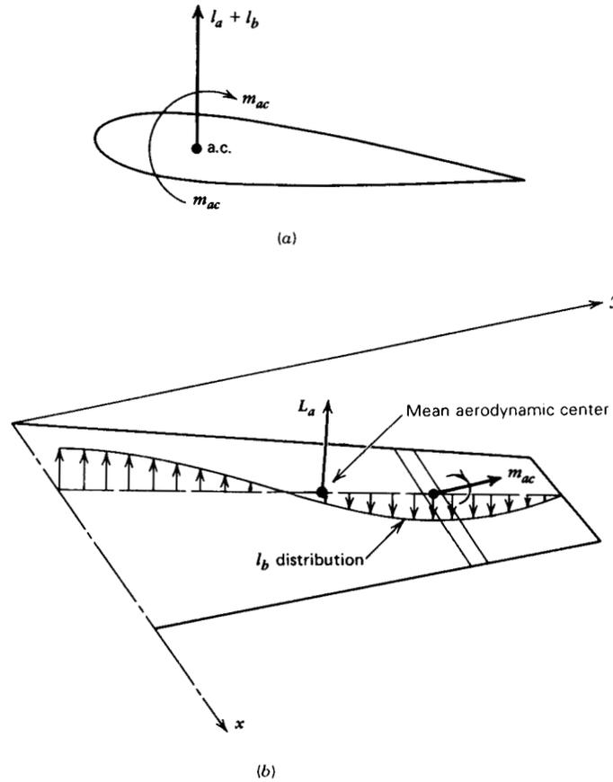
Figure C.4 (a) Section total load. (b) Wing loads.
