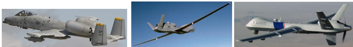
4. Fairchild A-10 Thunderbolt (H-tail) 5. Global hawk UAV (V-tail) 6. MQ-9 Reaper UAV (Y-tail) (Courtesy of Antony Osborne)
