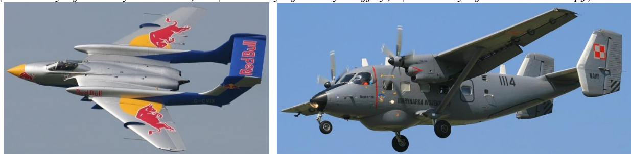
7. De Havilland DH-110 Sea Vixen (unconventional twin VT) 8. PZL-Mielec M-28 Bryza (H-tail) (Courtesy of Jenny Coffey) (Courtesy of Jenny Coffey)
