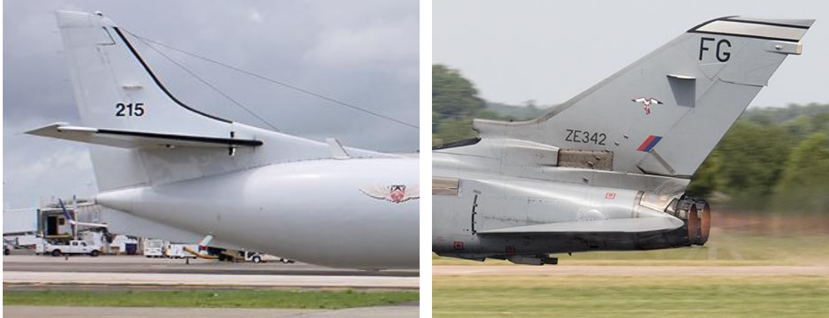
1. Adjustable horizontal tail in Fairchild C-26A Metro III (Courtesy of Luis David Sanchez) 2. All moving tail in Panavia Tornado (Courtesy of Antony Osborne) Figure 6.17. An adjustable tail and an all moving tail
