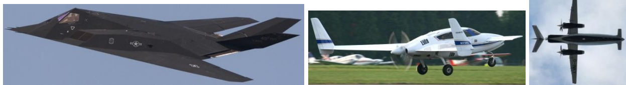
4. Lockheed F-117 Nighthawk (V-tail) 5. Velocity 173 Elite (canard and twin VT) 6. Piaggio P-180 (triplane) (Courtesy of Antony Osborne) (Courtesy of Jenny Coffey) (Courtesy of Hansueli Krapf)
