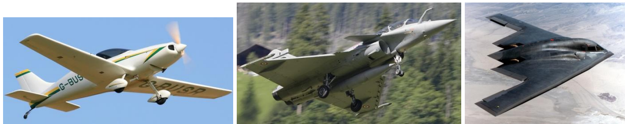
1. Aero Designs Pulsar (aft tail) 2. Dassault Rafale (canard) 3. B-2 Spirit (flying wing) (Courtesy of Jenny Coffey) (Courtesy of Antony Osborne)
