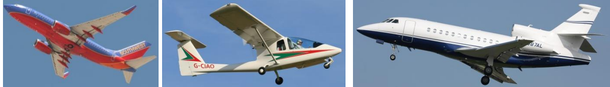
1. Boeing 737 (Conventional) 2. Sky Arrow 1450L (T-tail) 3. Dassault Falcon 900 (Cruciform) (Courtesy of Anne Deus) (Courtesy of Jenny Coffey) (Courtesy of Jenny Coffey)
