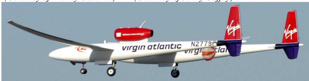
9. Global Flyer (unconventional tail); (Courtesy of NASA) Figure 6.12. Several aircraft with various aft tail configurations
