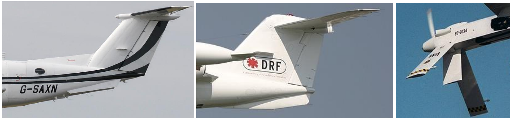
1. Beech 200 Super King Air (dorsal and ventral fin) 2. Gates Learjet 35A (ventral fin) 3. General Atomics Predator (ventral fin) (Courtesy of Jenny Coffey) (Courtesy of Antony Osborne)
