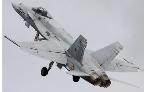
2. Applications of aileron, rudder, and elevator in a maneuver of a McDonnell Douglas EF-18 Hornet (Courtesy of Antony Osborne)
