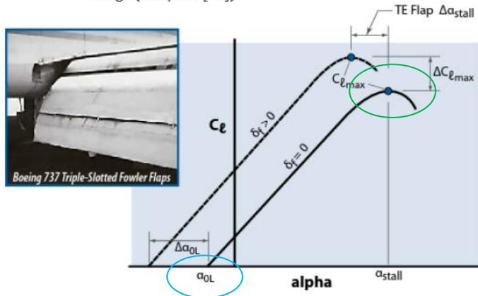
$$C_{L\alpha} = \frac{2\pi A}{2 + \sqrt{4 + \frac{A^2\beta^2}{\eta^2} \left(1 + \frac{\tan^2 \Lambda_{max,t}}{\beta^2}\right)}} \left(\frac{S_{exposed}}{S_{ref}}\right) (F)$$
