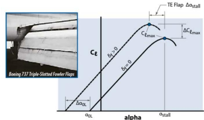
Figure 9.8 Construction of section lift curves for TE flaps.
