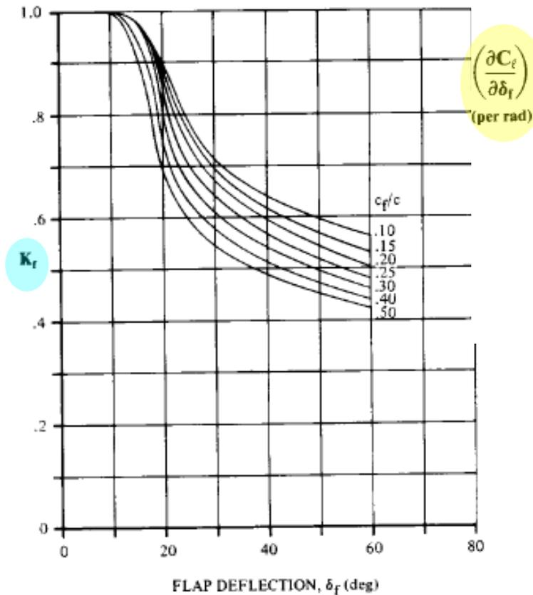
Fig. 16.7 Empirical correction for plain lift increment. (Ref. 37)
