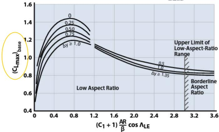
Figure 9.18 Subsonic maximum lift of low-AR wings (adapted [10]).
