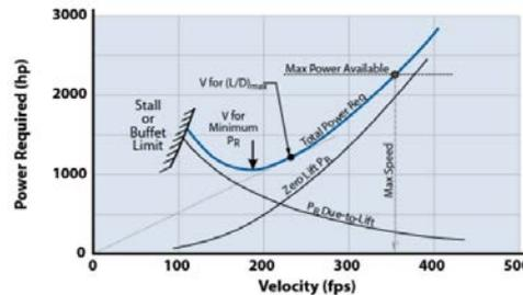
$$V_{\min \text{ power}} = \sqrt{\frac{2W}{\rho S}} \sqrt{\frac{K}{3C_{D0}}}$$
