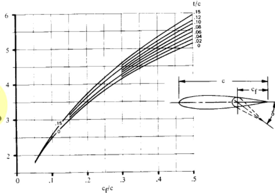
Fig. 16.6 Theoretical lift increment for plain flaps. (Ref. 37)
