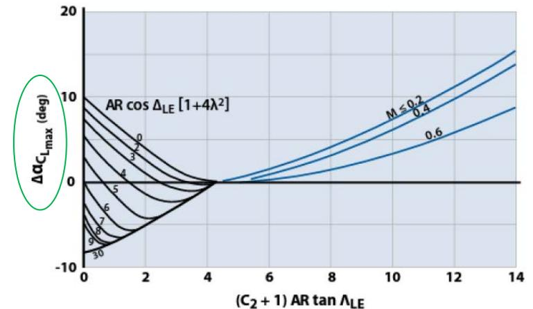
Figure 9.21 Angle-of-attack increment for subsonic maximum lift of low-AR wings.
