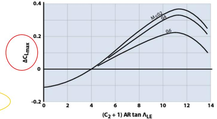
Figure 9.19 Subsonic maximum-lift increment for low-AR wings (adapted [10]).
