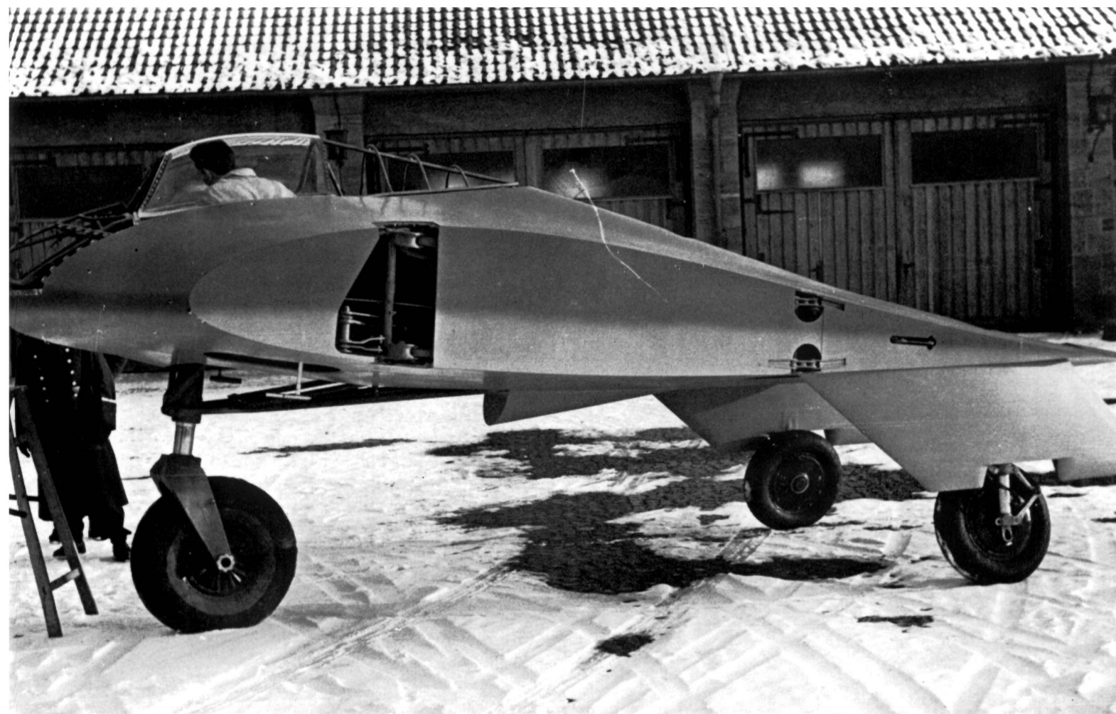
The main undercarriage was not retractable and was fitted with streamlined fairings to compensate for the stabilizing effect of the missing power plants. The aircraft's retractable nosewheel was in fact the tailwheel from a wrecked He 177 heavy bomber.
