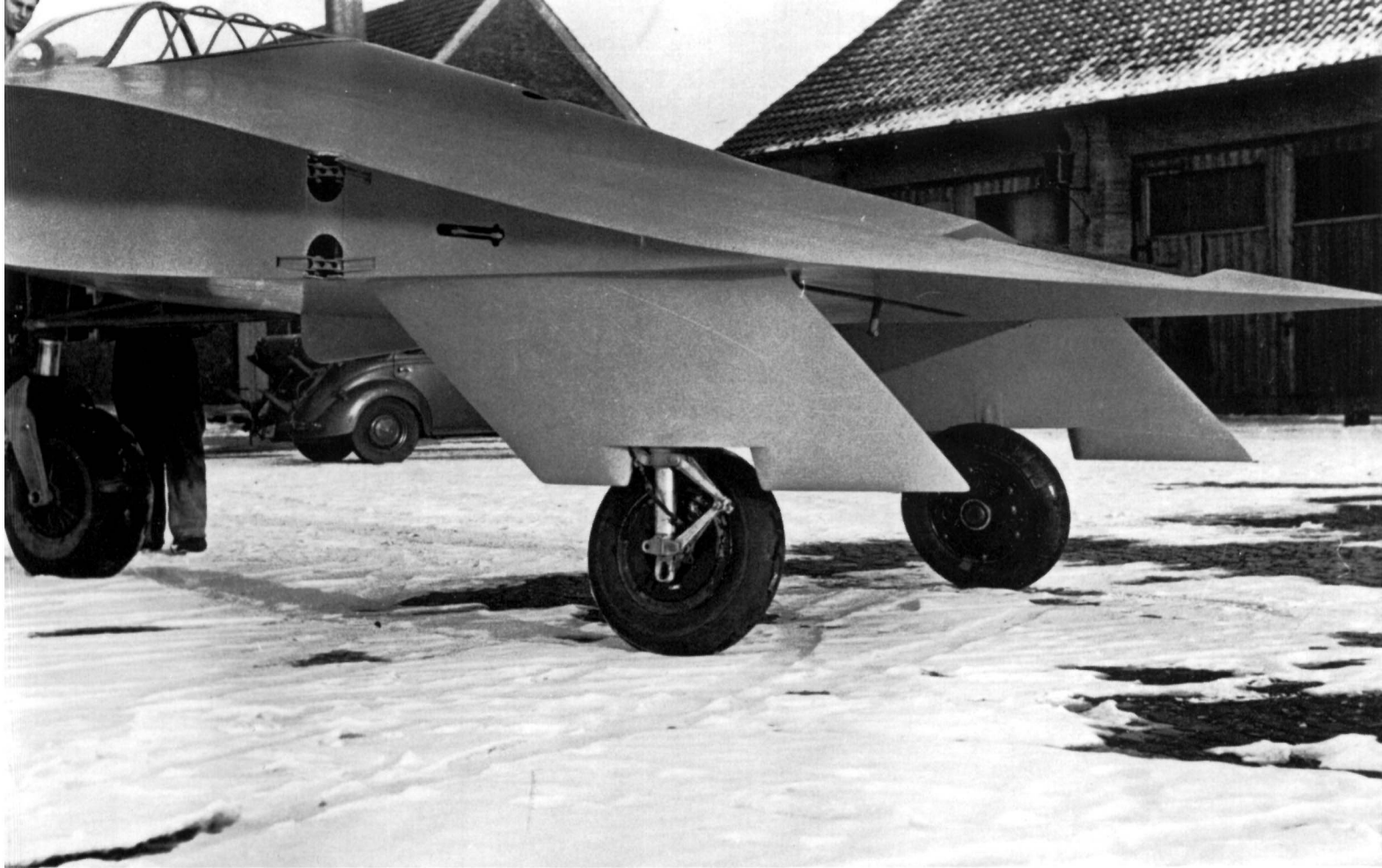
The main undercarriage was not retractable and was fitted with streamlined fairings to compensate for the stabilizing effect of the missing power plants. The aircraft's retractable nosewheel was in fact the tailwheel from a wrecked He 177 heavy bomber.
