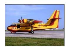
water. The CL-215 was first built in 1969 and was later replaced by the Bombardier 415 in 1994. These piston aircraft scoop water from lakes and reservoirs which can be dropped as regular water or be mixed with foam suppressant. The daily availability rate for the CL-215 is about \$9,100 per day with an hourly flight rate of about \$7,500 per hour.
